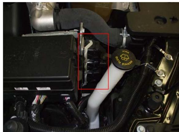
10) Determine which connector the **GREEN WOT Box Wire** goes to for your car with the pinout charts above. Remove enough of the loom behind this connector to access the wires. Splice the **GREEN WOT Box Wire** into the **WHITE** wire on the pin indicated on your vehicle's chart. Use the N2MB recommended soldering technique available at [www.n2mb.com](http://www.n2mb.com).
