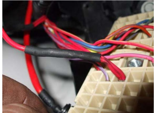
18) Join the **BLACK WOT Box Wire of the RED & BLACK Pair** to the wire end/ends going back into the harness. Here, the wire appears red on one side, but that's only the residue from separating the Red & Black Pair.
